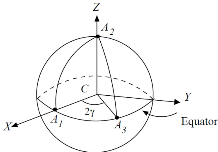
III.8. [1.5 mark] From figure it is clear that the area of the spherical triangle  $A_1A_2A_3$  is  $2\pi \times \left(\frac{2\gamma}{2\pi}\right) = 2\gamma$  and the phase difference was  $\gamma$ . Thus the phase difference is half the area of the spherical triangle  $A_1A_2A_3$  on Poincare sphere.
