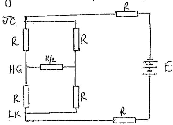
This is a balanced Wheatstone Bridge so  $R/2$  can be removed as no current flows through it.
