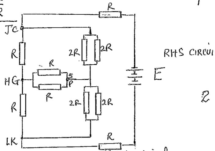
By symmetry circuits on either side of CGK (excluding CEK) identical. Hence S and P at same potential, so LHS circuit equivalent to RHS circuit above.
