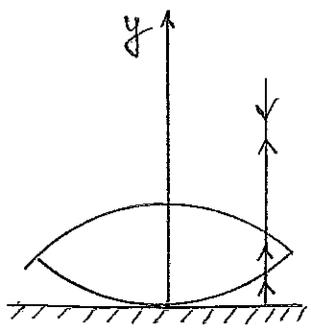
Monochromatic light incident normally on a convex lens, wavelength  $\lambda$ , sitting on an optical plate is partially reflected by the surface of the optical plate and the lower surface of the lens (see figure). These rays have a path difference and interfere. There is an extra phase difference of  $\pi$  produced by the optical plate. The circular symmetry about the  $y$ -axis gives rise to interference rings.
