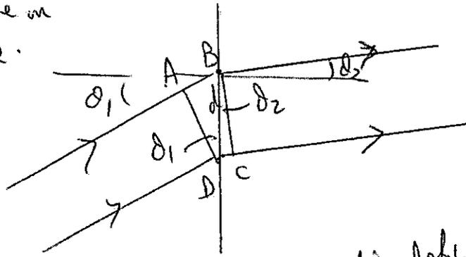
Separation of slits,  $d = \frac{1}{1.2 \times 10^6} \text{ m}$
