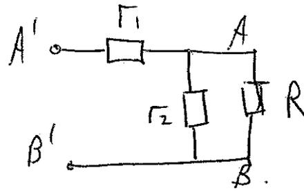
$$R_{A'B'} = \Gamma_1 + \frac{R\Gamma_2}{R+\Gamma_2}$$
