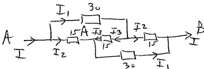
currents marked according to K.I. (and symmetry of the circuit).
