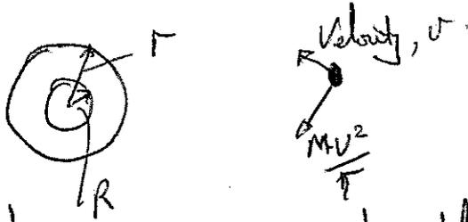
The force acting on the satellite is gravitational and given by  $\frac{GM_p \cdot m}{r^2}$ . Newton's 2nd law states that this unbalanced force is equal to  $F = ma$  with  $a = \frac{v^2}{r}$  for a circular orbit. Use of  $NII$  and gravity. ✓
