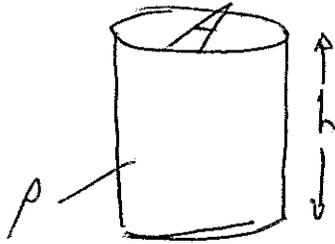
$$P_{\text{bottom}} = \frac{\text{force}}{\text{area}} = \frac{\text{weight}}{A}$$
