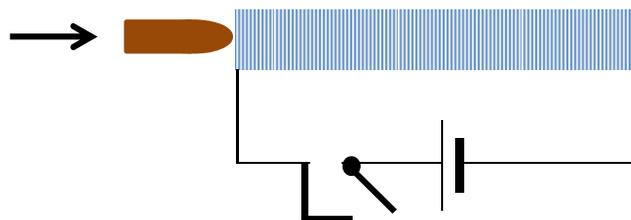
**Figure 4a.** Magnetic rifle (schematic)
