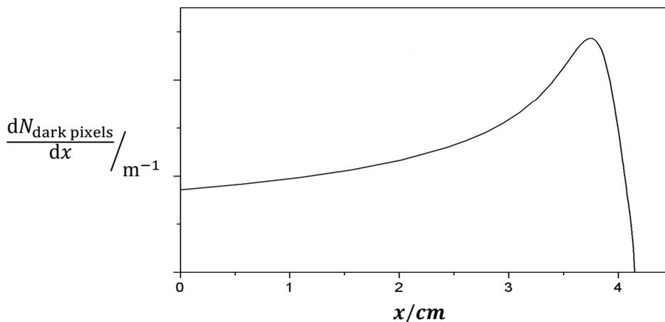
**Figure 1a.** Range of alpha particles in a gas when emitted by a source.
