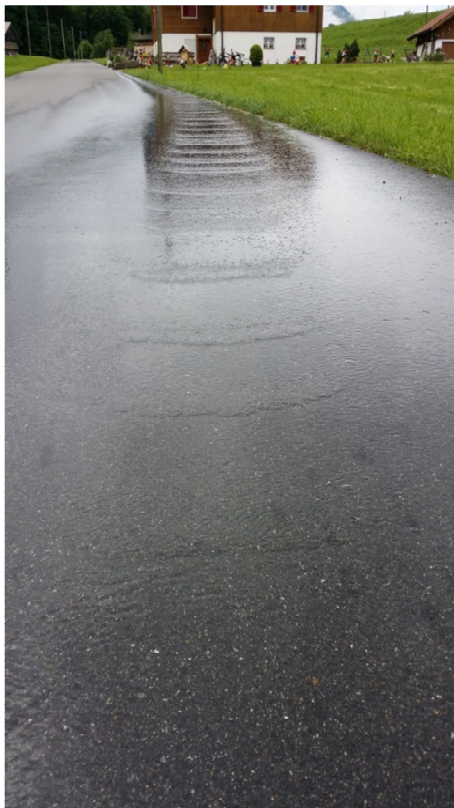
Figure 1.2 Flowing water on a shallow slope showing how the flow becomes uniform again when it spreads out.
