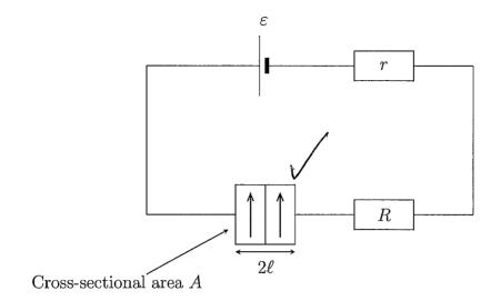
Considering either a spin-up or spin-down electron as it moves through these two layers, it experiences the same magnetisation throughout (either parallel or anti-parallel), for a total length of  $2\ell$ . Electrons with their spin parallel to the magnetic field will therefore experience a resistance of
