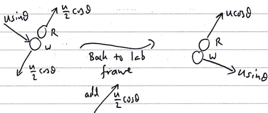
As White moves off after collision it has no velocity // to line of centres, while red moves only along line of centres. (Collision is assumed frictionless, so no force can be exerted on red in direction perpendicular to line of centres. Impulse only exerted // to line of centres so red must move off in that direction).
