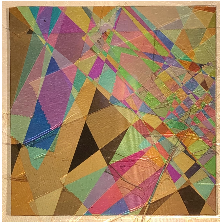
Figure 5: Sandwiched between two crossed polarisation filters, various strips of cellophane (sticky tape) have been set at random orientations, and are in places overlaying one another.
