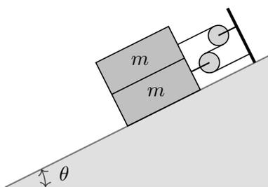
Suppose that the coefficient of static friction between the lower block and the slope is  $\mu$ , and all other surfaces are frictionless. What is the minimum value of  $\mu$  so that the blocks can stay static?
