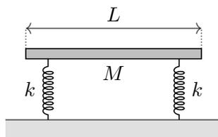
The rod is initially in equilibrium. If the rod is uniformly displaced downward and released from rest, what is the frequency  $f$  of its oscillations?
