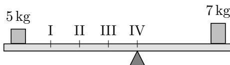
Two blocks, of masses 5 kg and 7 kg, are placed on the seesaw, so that it balances when the fulcrum is at point IV. (The diagram is not drawn to scale.) Now suppose the fulcrum is moved to point II. How much mass should be placed at point I so that the seesaw again balances?
