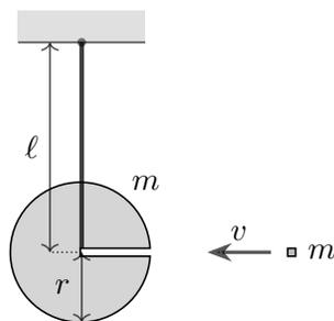
A uniform ball of mass  $m$  and radius  $r$  is attached to a massless rigid rod, so that its center is a distance  $\ell$  from the ceiling. The ball has a small tunnel hollowed out. A small block of mass  $m$  and speed  $v$  goes into the tunnel and collides at the center of the ball, perfectly inelastically. Subsequently, to what maximum height does the block rise?
