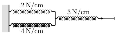
What force must be exerted at the end to extend the system by  $1\text{ cm}$  from its relaxed length?
