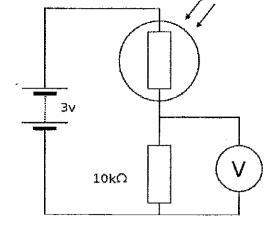
i) Show that, when the light level is 10 lux, the current in the circuit is 0.2 mA.
