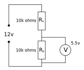
(c) Calculate the potential difference across the top resistor,  $R_{\text{A}}$ , with the voltmeter connected as shown in the diagram above.
