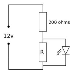
If the LED requires an operating voltage of 2 volts and a current of 20 mA, calculate a suitable value for the unknown resistor R.
