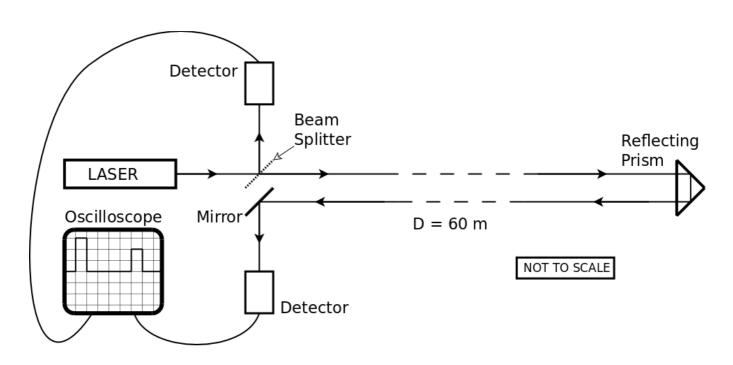
The timebase on the oscilloscope is set to 0.1  $\mu s$  per division.
