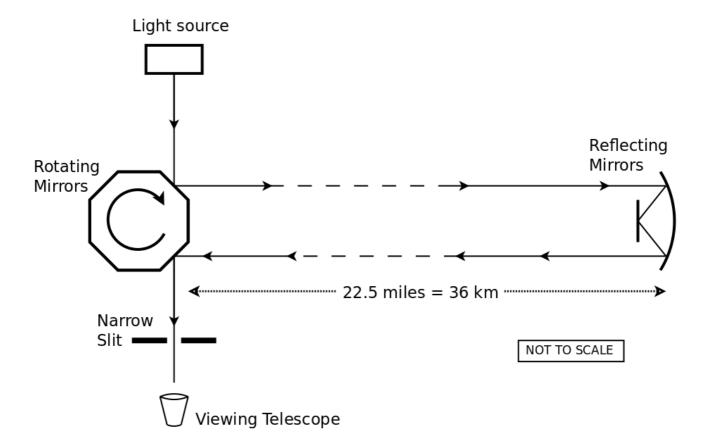
A narrow light beam from the source was reflected off one face of the rotating mirror, travelled to an adjacent mountain top 36 km away and returned to be observed through the telescope, as shown.
