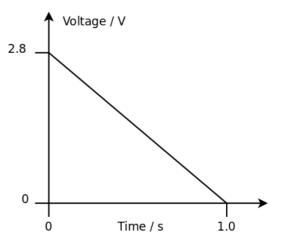
As the supercapacitor discharges, the voltage reduces steadily from 2.8V to 0V as shown on the voltage – time graph.
