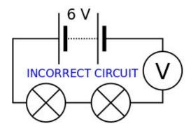
A second student uses the same components but rebuilds the circuit **incorrectly** with all three components in series.
