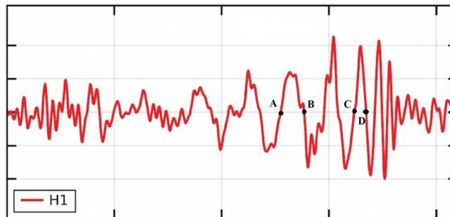
Figure 1. Strain, i.e. relative variation of the size of each arm, at the LIGO detector H1. The horizontal axis is time, and the points A, B, C, D correspond to  $t = 0.000, 0.009, 0.034, 0.040$  seconds, respectively.
