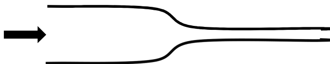
Figure 1. Incompressible liquid flowing through a tube which narrows.
