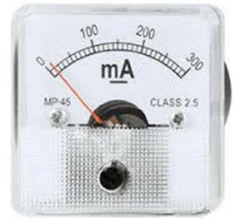
Figure 4. Typical moving coil meter.
