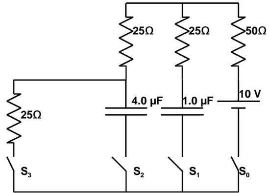
**(a, 5)** Switches  $S_0, S_1, S_2$  are closed. Switch  $S_3$  remains open. After a very long time, what is the charge on each capacitor?
