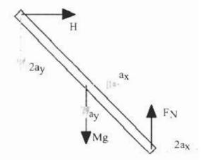
c. Considering both rods as the system so we don't need to include the work done by the forces H and V,  $PE_{Li} + PE_{Ri} = PE_{Lf} + PE_{Rf} + KE_{Lf} + KE_{Rf}$  (c.1)
