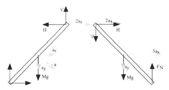
Bla.. For  $\theta = 45^\circ$ , both  $\cos\theta = 1/\sqrt{2}$  and  $\sin\theta = 1/\sqrt{2}$ . The relation between the magnitude of the angular acceleration  $\alpha$  and the magnitude of the linear acceleration  $\alpha$  is  $a = \alpha L/2$  with  $a_x = a_y = \alpha L/(2\sqrt{2})$ . Using  $I\alpha = \Sigma \tau$  for the rotation about the hinge at the lower end of the left rod
