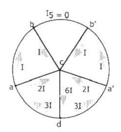
This is the emf induced in the circuit branch cd. By symmetry the currents to the left of cd equal those to the right of cd.  $I_5 = 0$ . Since no current branches off at b,  $I_4 = I_3 = I$ . The potential drop between point points a and c must be independent of path, so
