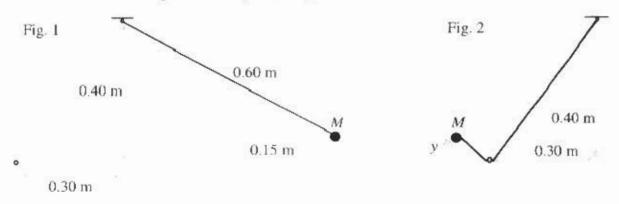
(15) a. Find an expression for the tension T in the string when the string is in contact with the rod. (10) b. Find the x- and y-components of the force that the rod exerts on the string.
