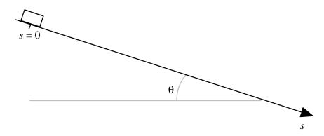
1. A small block of weight mg is initially at rest at the starting point s = 0 shown above. It slides down an increasingly rough incline at an angle of  $\theta$  to the horizontal. The coefficient of kinetic friction is
