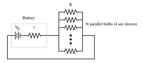
The battery is connected to N identical lightbulbs in parallel. The bulbs each have a fixed resistance R, independent of the current through them.
